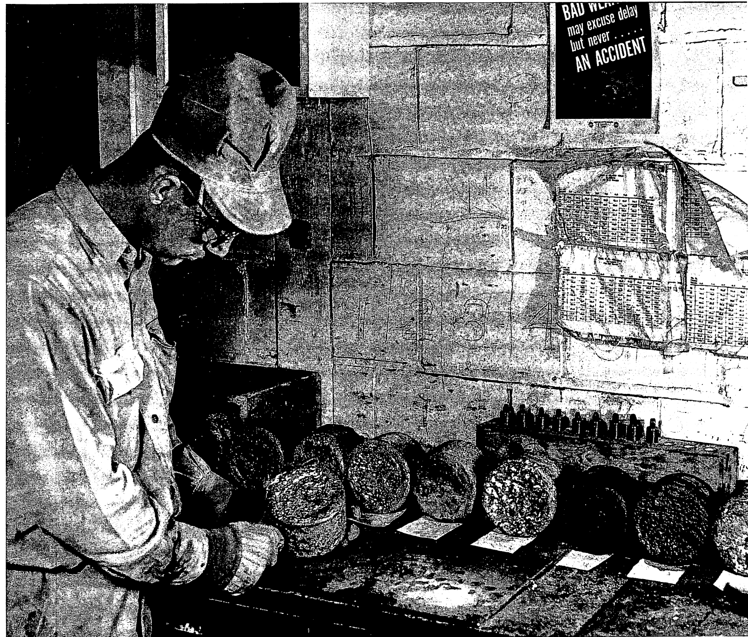
The uranium reduction process at the Ames Project yielded "biscuits" that could be cast into ingots.
